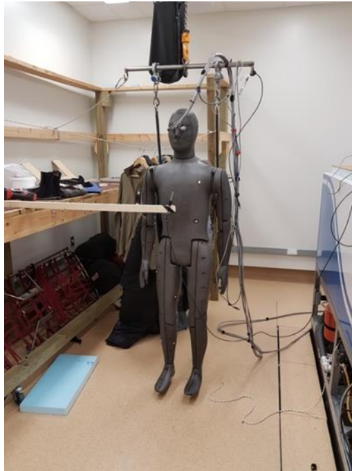
Figure 1: Thermal manikin, NEMO, in NRC-OCRE's TML.
