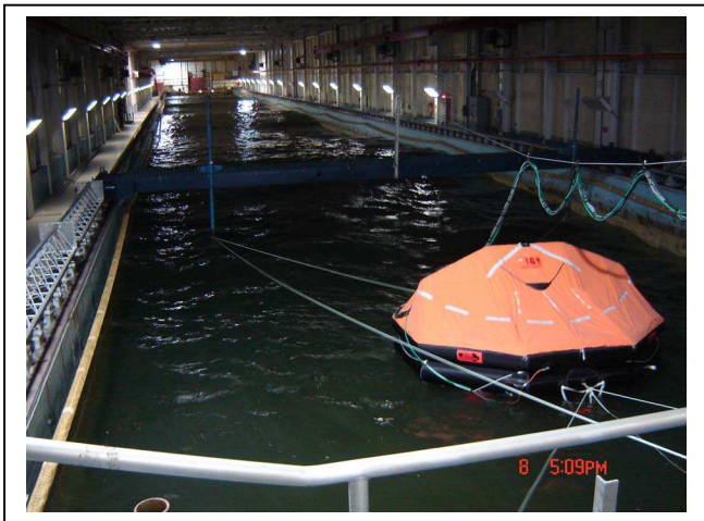
Figure 1. Life raft setup between the towing carriage and the service carriage in Phase 1
