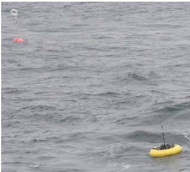
**Figure 7: Directional Wave Buoy**
