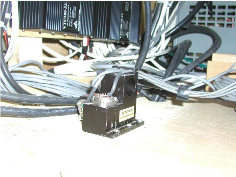
**Figure 5: Orthogonal Linear Accelerometers on Bridge**
