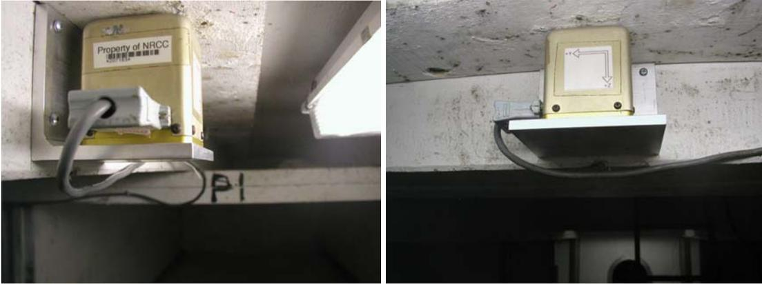
**Figure 4: MotionPak Installation in Fish Hold**
