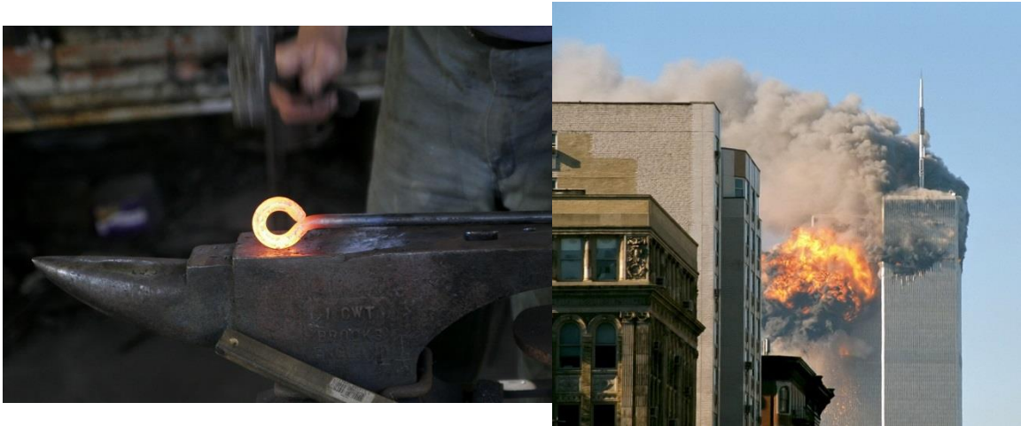
Figure 10: Two examples of materials at a high homologous temperature: Left) A red hot iron rod being hammered into shape. 1 ; Right) Some critical steel components in the WTC twin towers' structure in New York, whose failure ultimately caused domino-style floor collapse. 2
