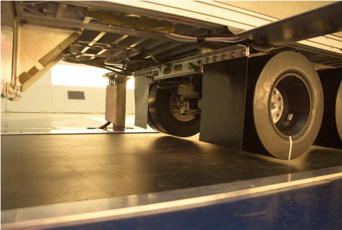
Figure E.5: Model modifications in 2015: trailer mud flaps.
