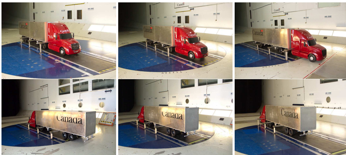
Figure D.1: Sleeper-cab tractor with 40 ft trailer: aft model location (left), mid model location (centre), and forward model location (right).
