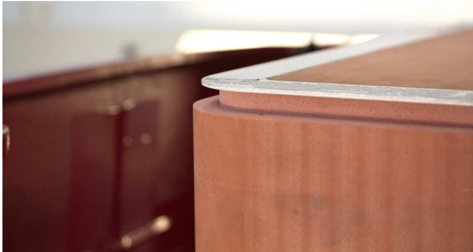
Figure E.3: Model modifications in 2015: trailer roof-edge drip rail.
