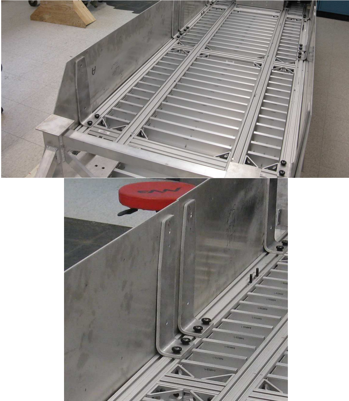
Figure A.3: The wind tunnel model of the NRC Trailer Skirts. The skirts are shown installed on the bottom of the overturned model trailer (top) with a close-up view of the mounting brackets (bottom).
