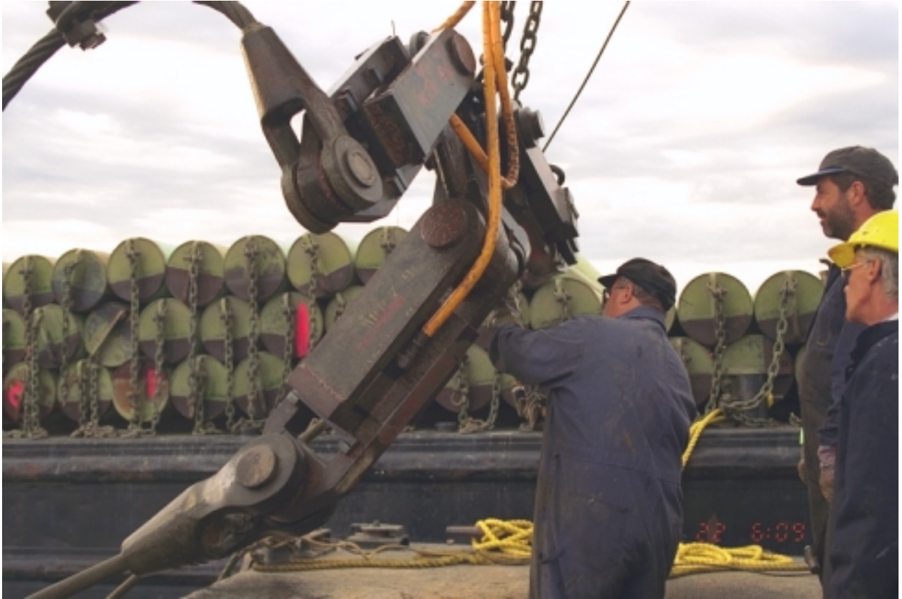
Figure 8.4 Typical load cell deployment at Yamachiche boom
