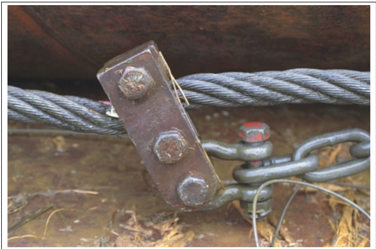
Figure 8.1 Cable clamp twisting a section cable
