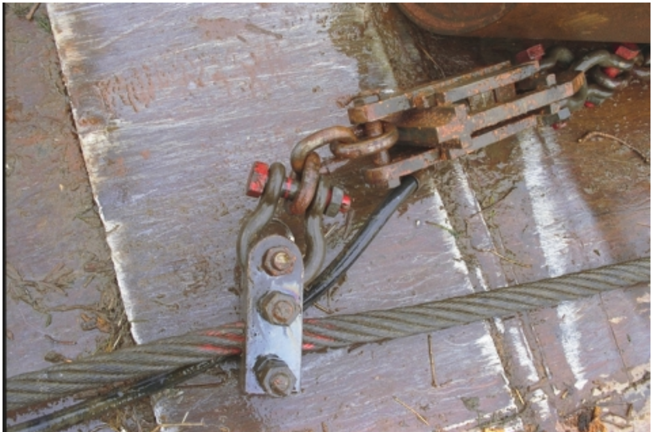
Figure 8.2 Very small cage deployed on chain between pontoon and section cable
