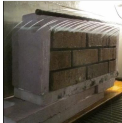
Figure 23 – Unidirectional freeze-thaw chamber during a thaw cycle with a wall panel installed
