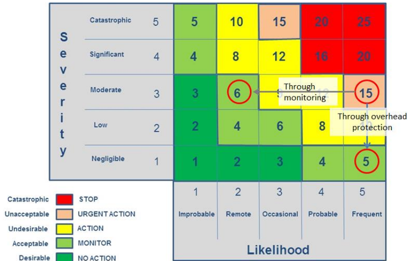
Figure 34 – Example of qualitative risk grid and examples of actions considered to mitigate identified risk factor and permit moving to lower risk level
