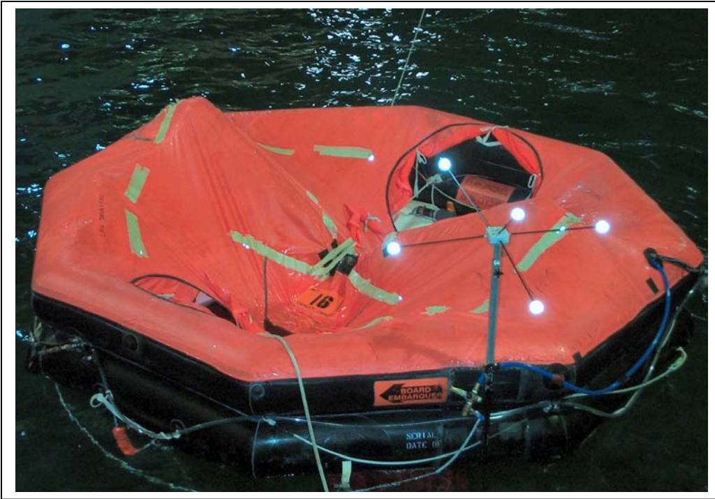
Figure 6.44 A puddle of water remained on the collapsed canopy.
