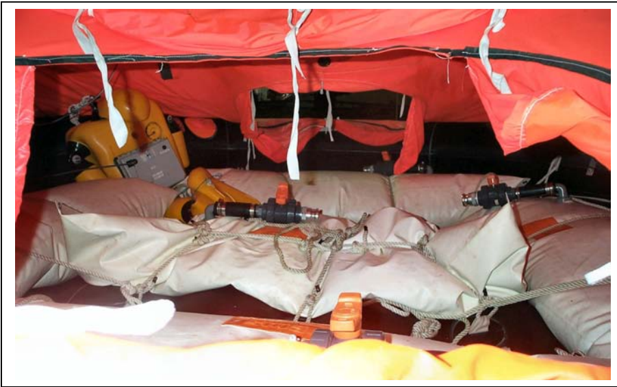
Figure 5.3 Life raft with water ballast bags (even weight distribution)
