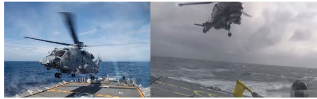
Fig. 2. Ship-helicopter operations on a stern flight-deck. Left side: low sea state (Skies Magazine, 2019), right side: high sea state (Society of Rock, 2020).
