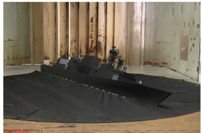
Fig. 10. Downstream view of 1:50 scaled ship in maximum roll position in the 3 m × 6 m Wind Tunnel.
