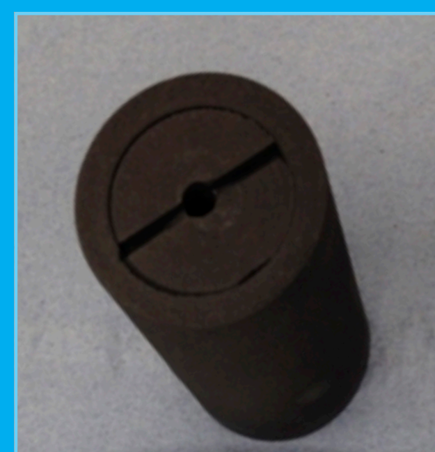
Figure 2: A high temperature fixed-point blackbody
