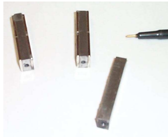
Figure 5. Flux concentrators made of SMC material with process B. Two of them have magnets mounted on their sides.
