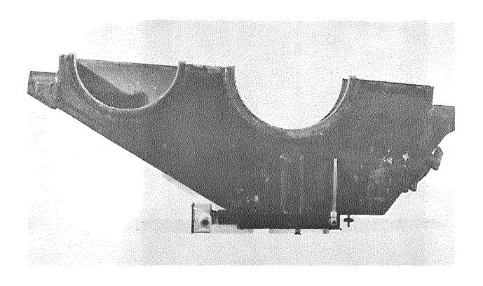
FIG. 1 STEEL GEAR CASE FITTED WITH WATER SUMP AND 3 kW ELECTRIC HEATER
