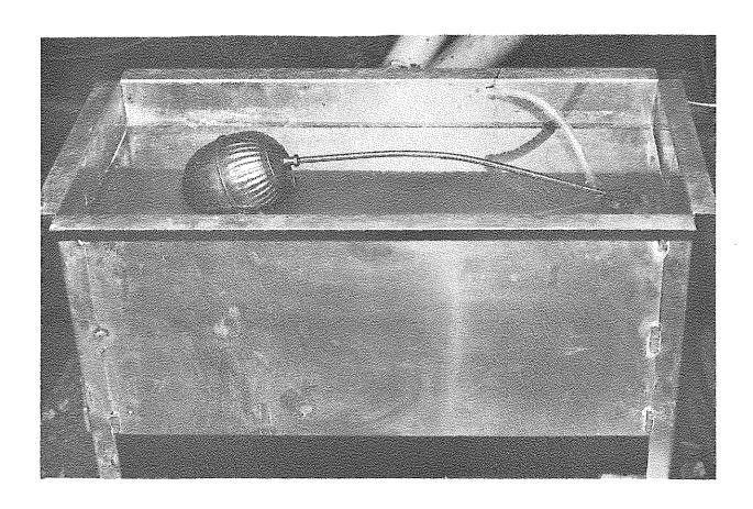
FIG. 2 WATER RESERVOIR WITH FLOAT LEVEL CONTROL
