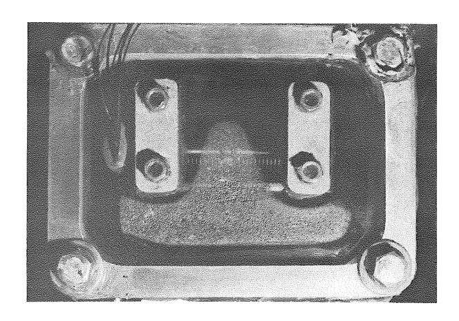
FIG. 4 CONDENSATE ON WINDOW OF COMMUTATOR END OIL RESERVOIR
