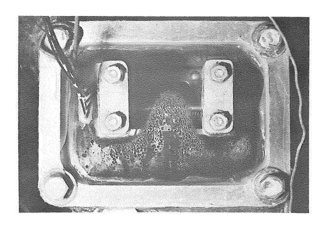
FIG. 5 CONDENSATE ON WINDOW OF PINION END OIL RESERVOIR
