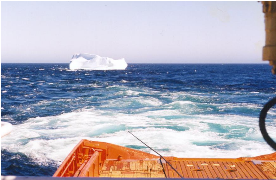
Figure 2.11 Iceberg Towing by Normand Jarl
