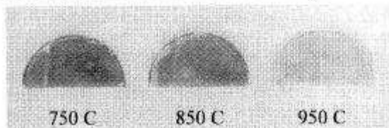
Figure 2. Photograph of composite cathodes fired at various temperatures remaining on scotch tape.
