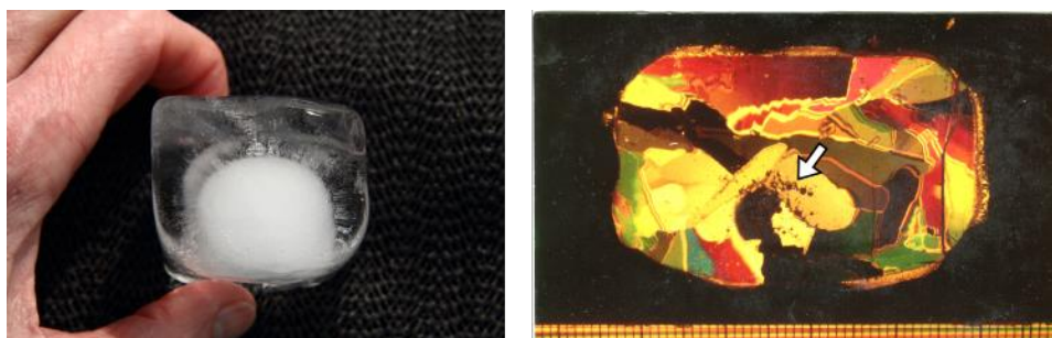
Figure 1: Left) A standard ice cube – the white zone in the center is where tiny air entrapments have developed during freeze-up. Right) Thin section of an ice cube – the various colors are the crystals (the white arrow points to the largest air entrapments – the smaller ones are not visible under these light conditions). The scale at the bottom right is in millimeters.
