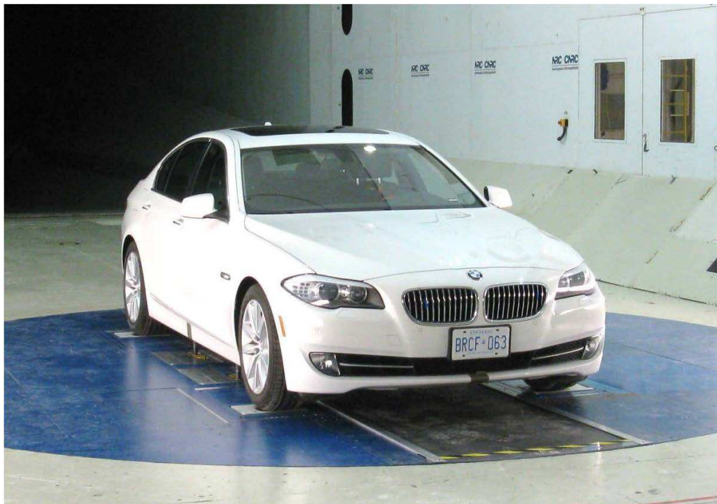
Figure B.1: View from upstream of the 2013 BMW 528i on the GESS in the 9 m Wind Tunnel.
