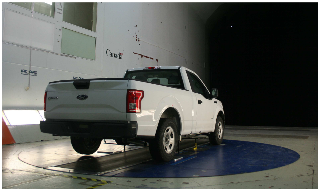
Figure 2.4: View of a pick-up truck installed on the GESS with the rear wheels suspended above the tunnel floor.
