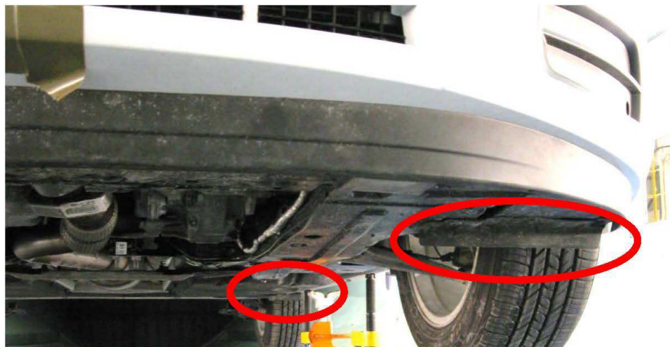
(a) Bumper air dam (foreground) and wheel dams (circled in red)
