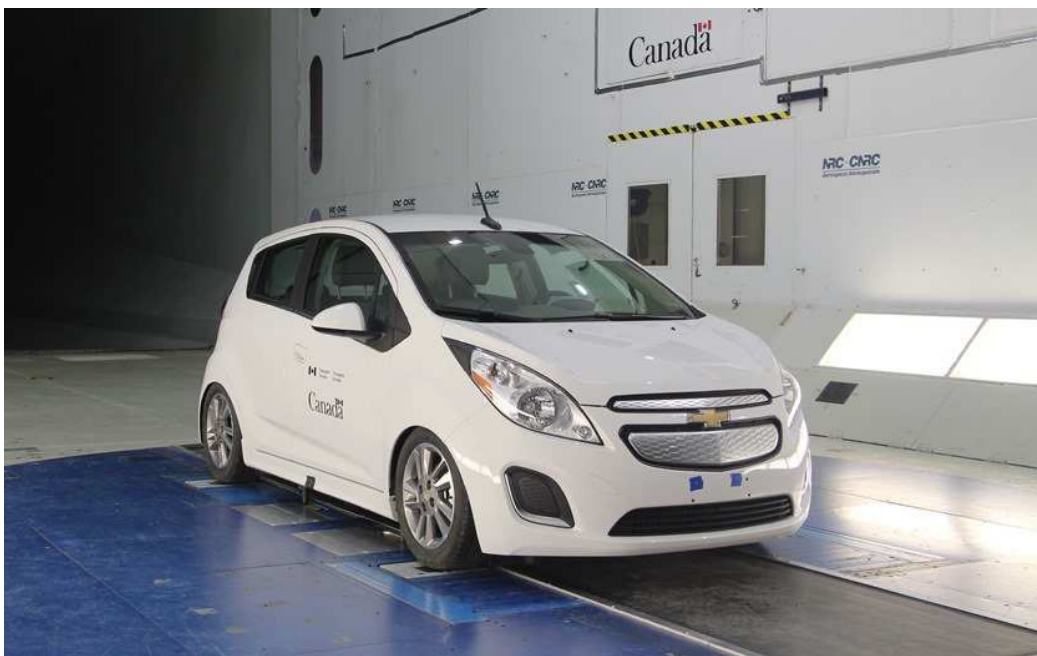
Figure B.14: View from upstream of the 2014 Chevy Spark EV on the GESS in the 9 m Wind Tunnel.
