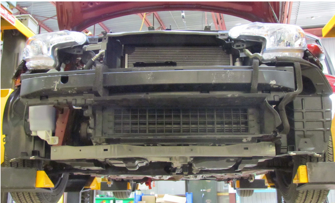
Figure 2.7: View of the front end of a vehicle with the front fascia removed. The lower radiator is equipped with AGS, seen in the fully opened position in the picture.
