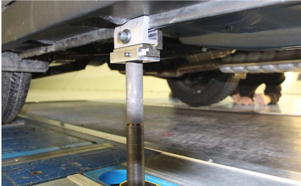
Figure 2.3: Close-up view of a rear GESS strut and rear GESS clamp attached to the rocker panel of a SUV.
