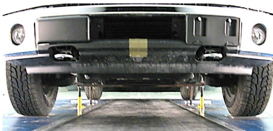
(d) Front view of vehicle with OEM bumper air dam
