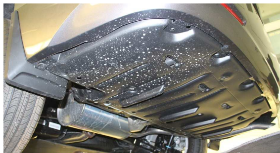
(b) Vehicle with smooth OEM rear underbody panel
