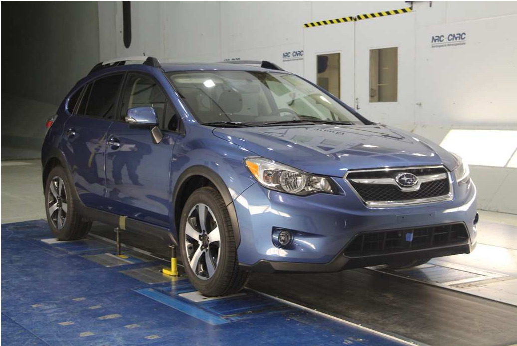
Figure B.11: View from upstream of the 2014 Subaru Crosstrek on the GESS in the 9 m Wind Tunnel.
