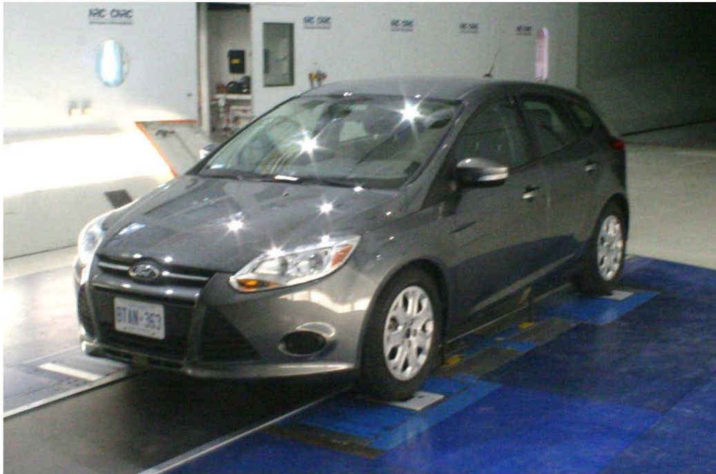
Figure B.5: View from upstream of the 2013 Ford Focus on the GESS in the 9 m Wind Tunnel.
