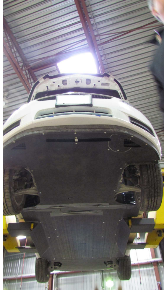
(b) Prototype, smooth underbody panels
