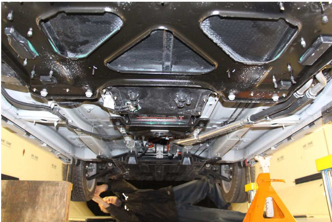
(b) Vehicle underbody with OEM panels removed
