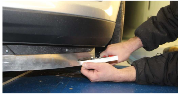
(b) Adjusting the extended OEM air dam
