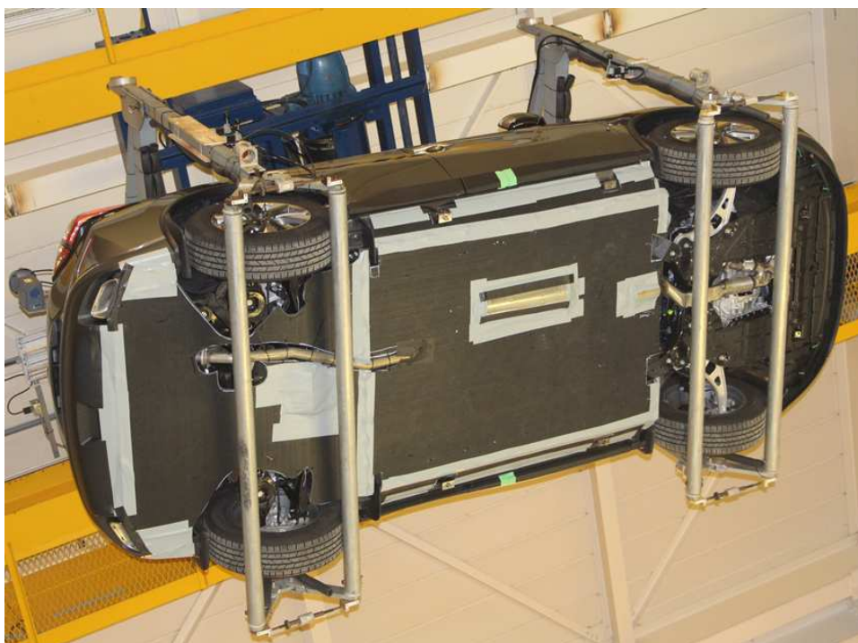
Figure 3.23: Views from below of the underbody of a vehicle completely covered with custom panels, with the exception of the covering of the engine compartment which is a standard OEM part. (Picture taken during the lifting process of the vehicle in the test section of the 9 m Wind Tunnel).
