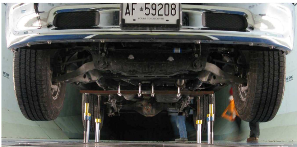
(b) Mounts on a pick-up truck with the struts in the raised position.
