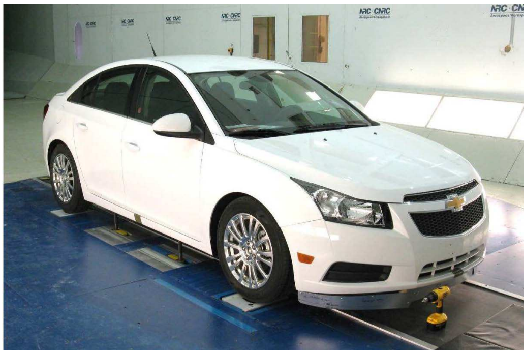
Figure B.2: View from upstream of the 2014 Chevrolet Cruze on the GESS in the 9 m Wind Tunnel.
