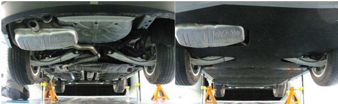
(b) Vehicle with OEM underbody panels (left) and custom underbody panels (right)
