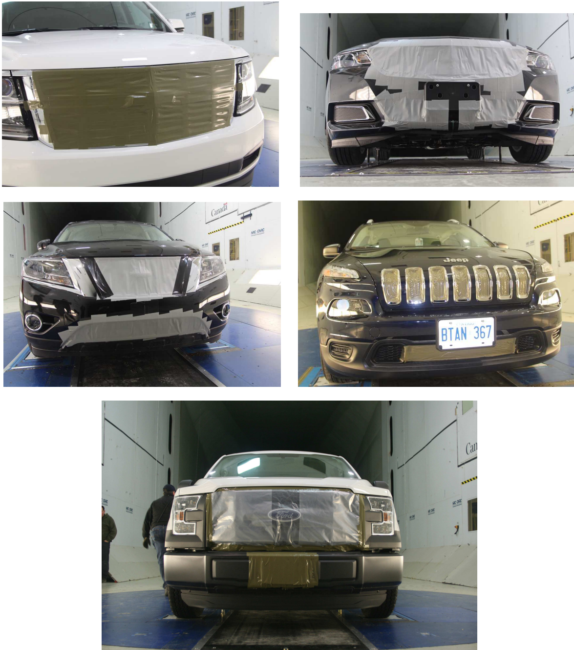
Figure B.28: Examples of vehicles with external grille sealed.
