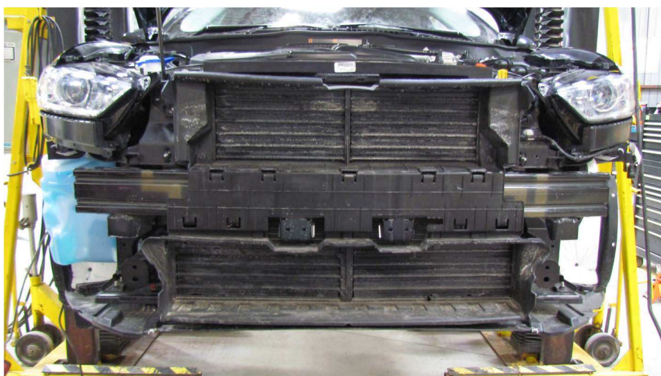
(c) Upper and lower grille shutters (closed), front fascia removed.
