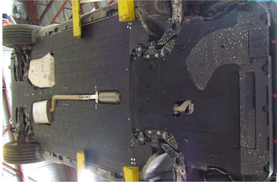
(a) Vehicle with OEM underbody panels at front and custom underbody panels at rear
