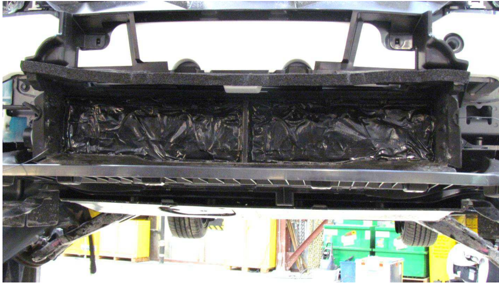
Figure 2.10: AGS unit taped shut, revealed by bumper removal.
