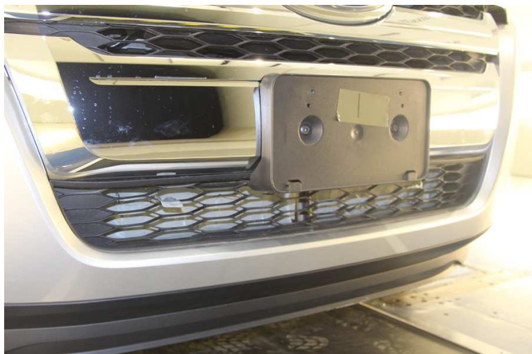
(c) Vehicle with AGS on lower radiator sealed
