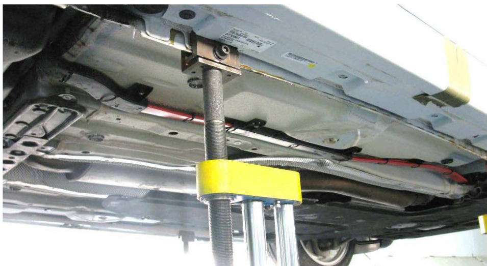
(a) Rocker panel clamps installed on a vehicle.
