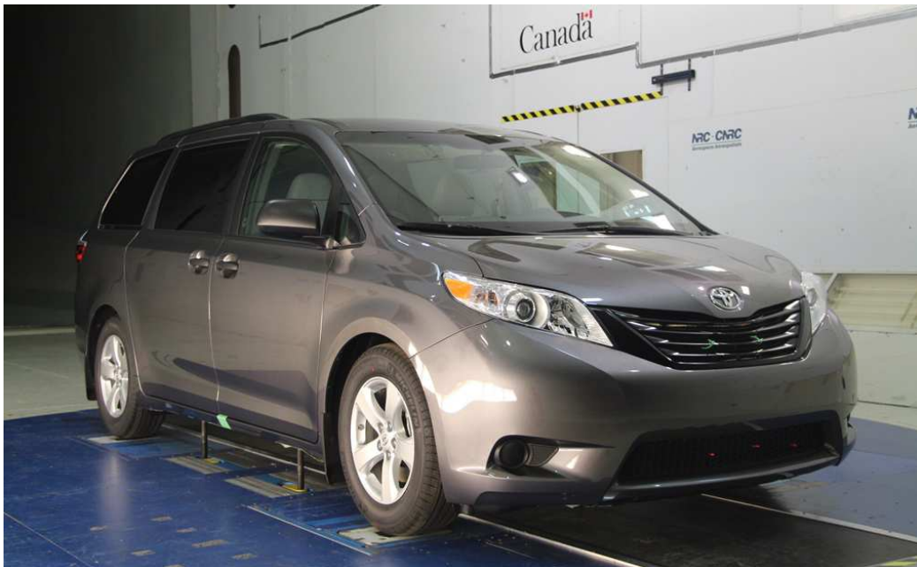
Figure B.22: View from upstream of the 2015 Toyota Sienna on the GESS in the 9 m Wind Tunnel.
