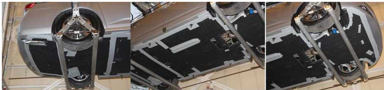
(c) Rear (left), middle (center) and front (right) custom underbody panel sections on a vehicle
