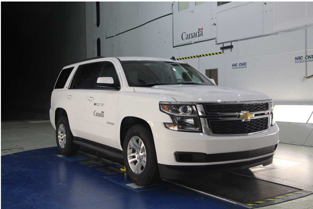
Figure B.16: View from upstream of the 2015 Chevy Tahoe on the GESS in the 9 m Wind Tunnel.
