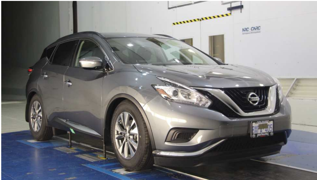
Figure B.21: View from upstream of the 2015 Nissan Murano on the GESS in the 9 m Wind Tunnel.
