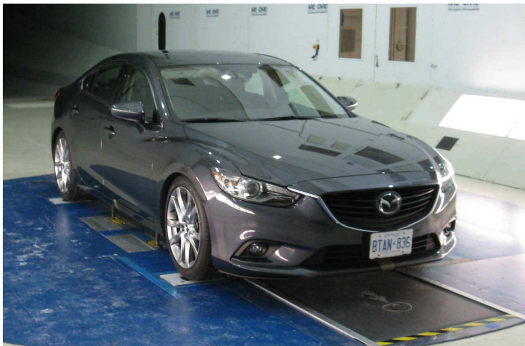
Figure B.8: View from upstream of the 2014 Mazda 6 on the GESS in the 9 m Wind Tunnel.
