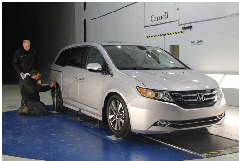
(c) Adjusting the rear ride height of a vehicle
