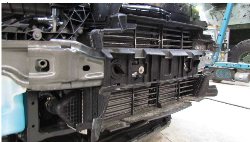
(b) Upper and lower grille shutters (open) with front fascia removed
