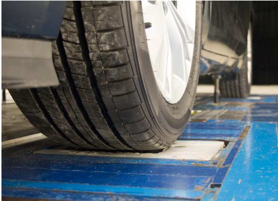
Figure 2.5: Close-up view of a light-duty vehicle wheel and GESS wheel roller in the 9 m Wind Tunnel.
