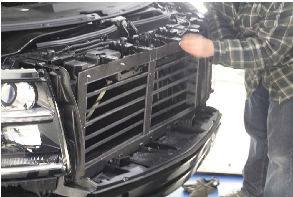
Figure 2.9: View of the mock-up AGS frame built at NRC by Röchling Automotive, front bumper removed.
