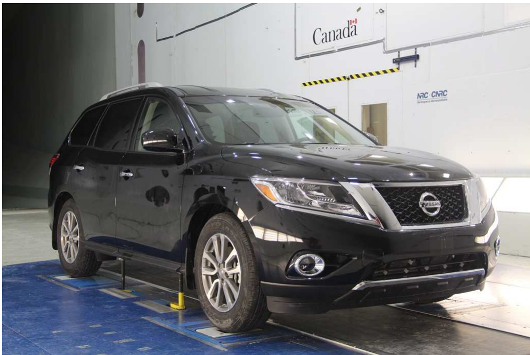
Figure B.18: View from upstream of the 2015 Nissan Pathfinder on the GESS in the 9 m Wind Tunnel.
