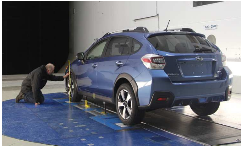
(a) Adjusting the front ride height of a vehicle
