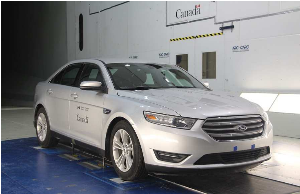
Figure B.15: View from upstream of the 2014 Ford Taurus on the GESS in the 9 m Wind Tunnel.
