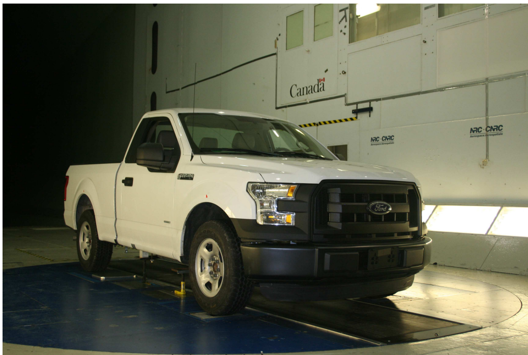
Figure B.23: View from upstream of the 2016 Ford F-150 on the GESS in the 9 m Wind Tunnel.
