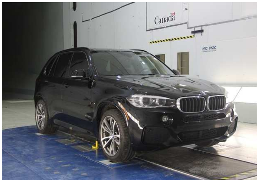
Figure B.10: View from upstream of the 2014 BMW X5 on the GESS in the 9 m Wind Tunnel.
