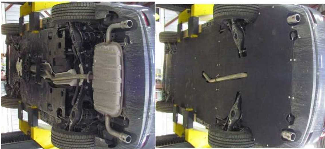
(c) Vehicle with OEM underbody panels (left) and custom underbody panels (right)
