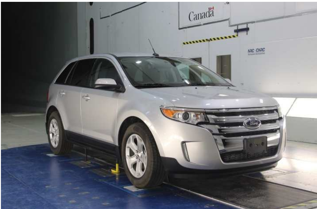
Figure B.12: View from upstream of the 2014 Ford Edge on the GESS in the 9 m Wind Tunnel.
