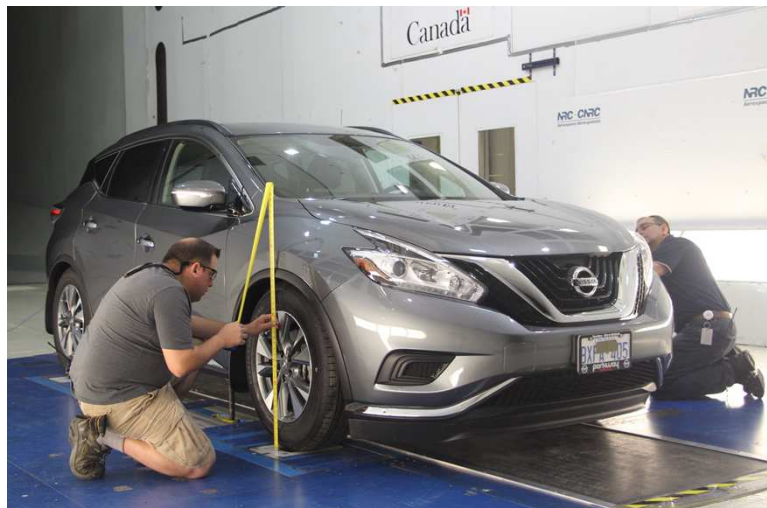
(b) Adjusting the front ride height of a vehicle
