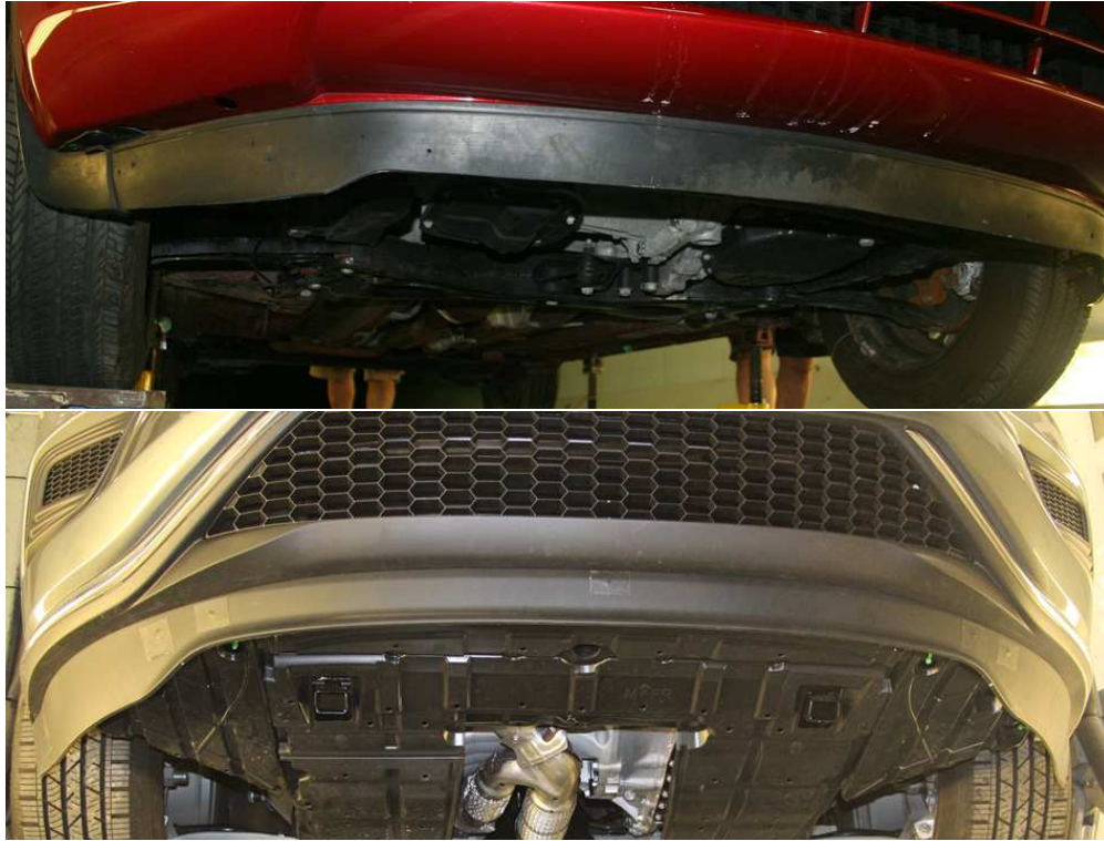
Figure 2.12: Close-up views of OEM bumper air dams.
