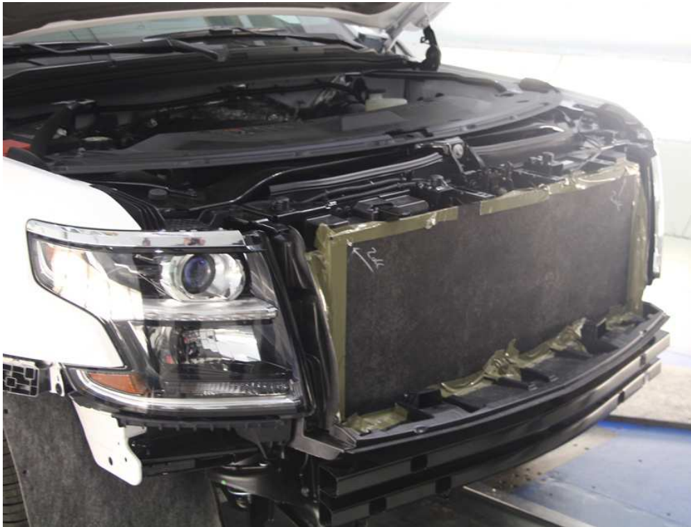
Figure 2.8: View of the solid panel covering the radiator and part of the custom AGS built at NRC by Röchling Automotive, front bumper removed.
