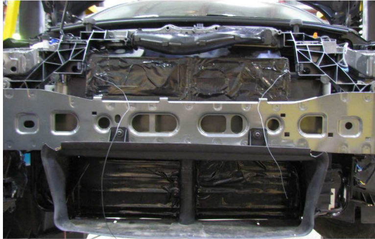
(a) Vehicle with grille shutters taped, front fascia removed.
