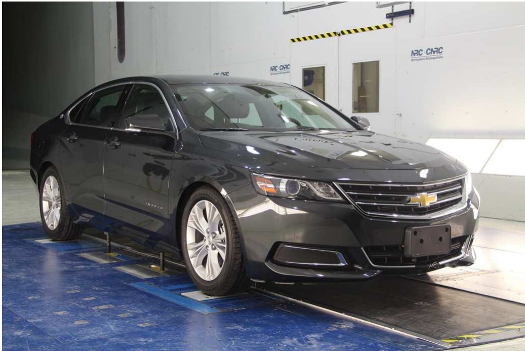
Figure B.17: View from upstream of the 2014 Chevy Impala on the GESS in the 9 m Wind Tunnel.
