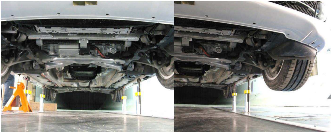
(a) Vehicle underbody with OEM panels removed
