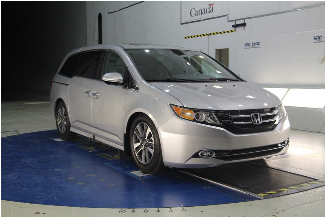
Figure B.13: View from upstream of the 2014 Honda Odyssey on the GESS in the 9 m Wind Tunnel.
