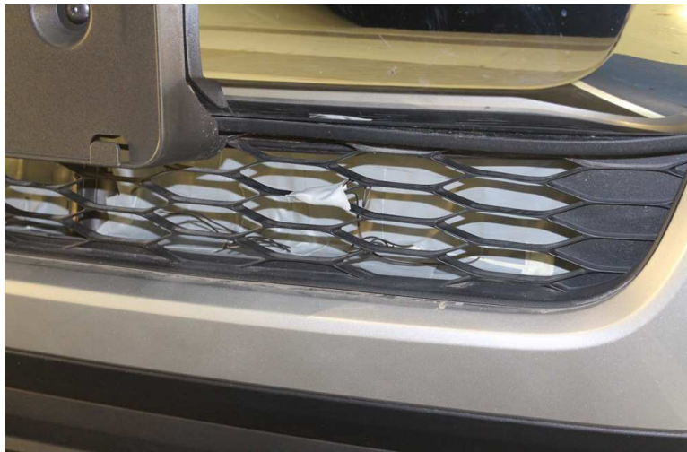
(b) Vehicle with AGS on lower radiator sealed
