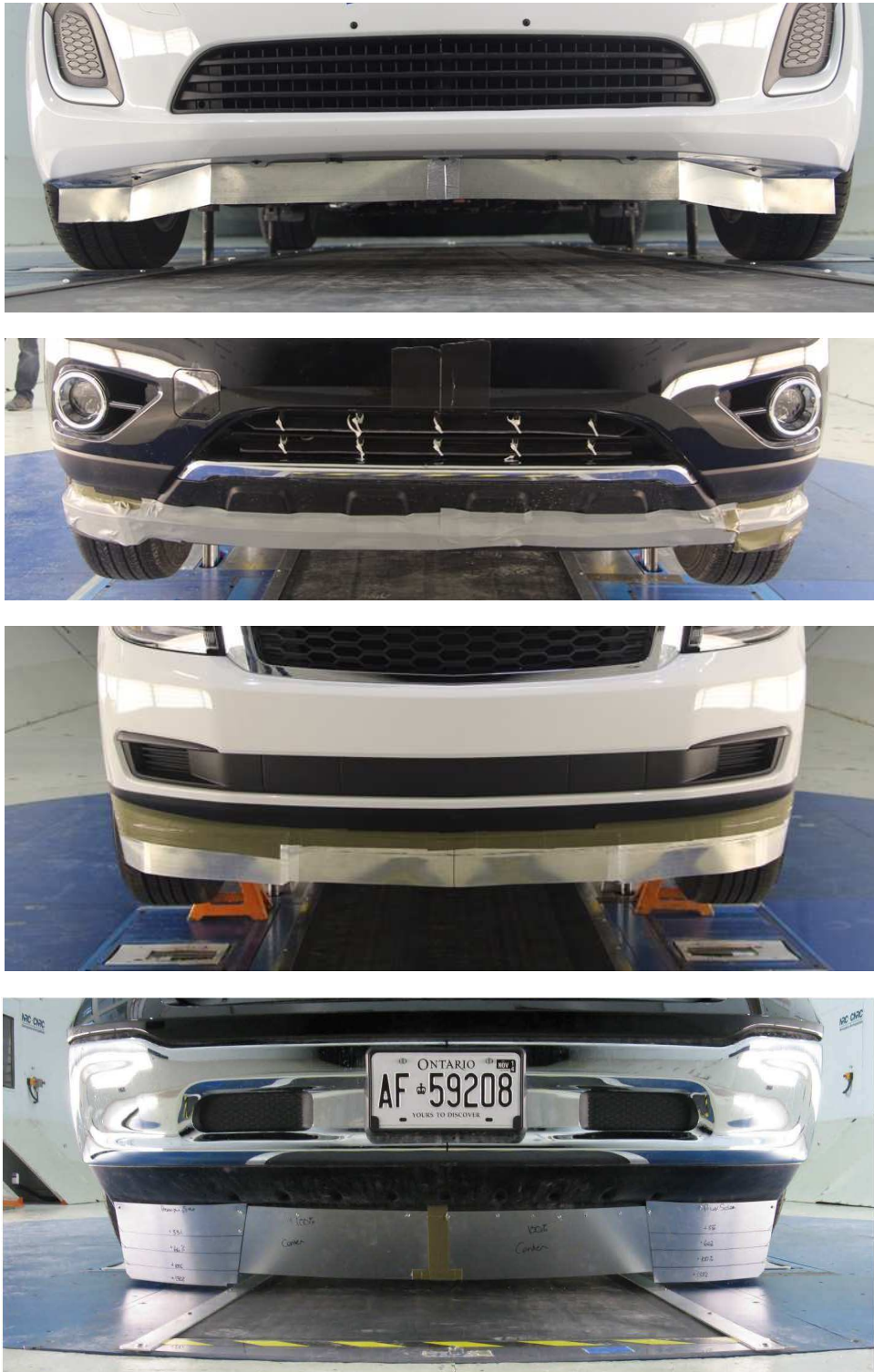
Figure B.37: Examples of vehicles fitted with custom-built bumper air dams.
