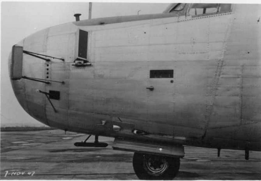
CAMERA INSTALLED ON AIRCRAFT
