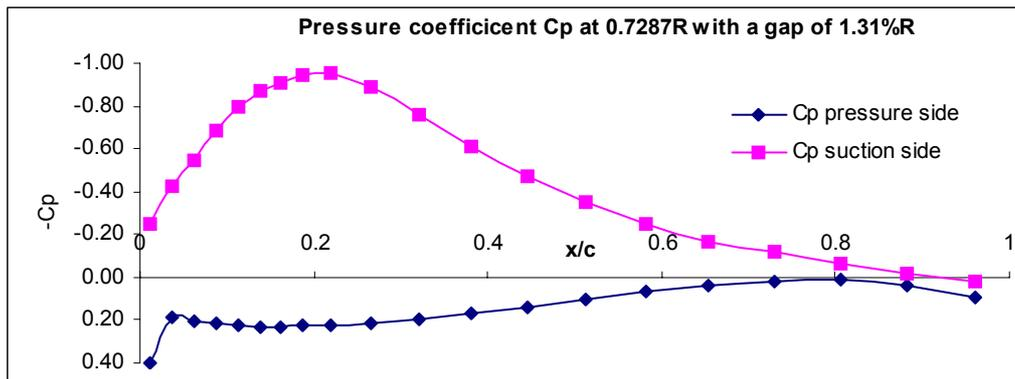
Figure 9: Pressure distribution of the key blade at the 179<sup>th</sup> time step (1.31%R) at a radial location of  $r=0.7287R$ .
