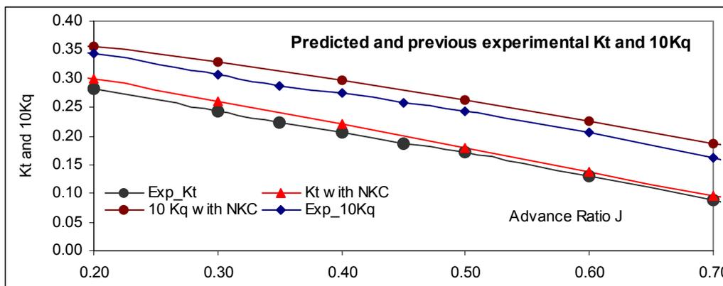
Figure 3: Validation of the prediction by the current method and the previous experimental results in a wide range of load conditions from  $J=0.2$  to  $0.7$  which correspond to the load factor of from  $J/[p/D]=0.256$  to  $0.897$
