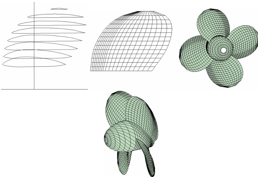
Figure 1: Sectional shape panel layout of the ice class propeller in expanded plan and the rear and side views of this propeller. The pitch ratio at  $r=0.7R$  is  $0.78$  and the hub to diameter ratio is  $0.30$ . This propeller has a rake angle of  $10^\circ$  and minor skew
