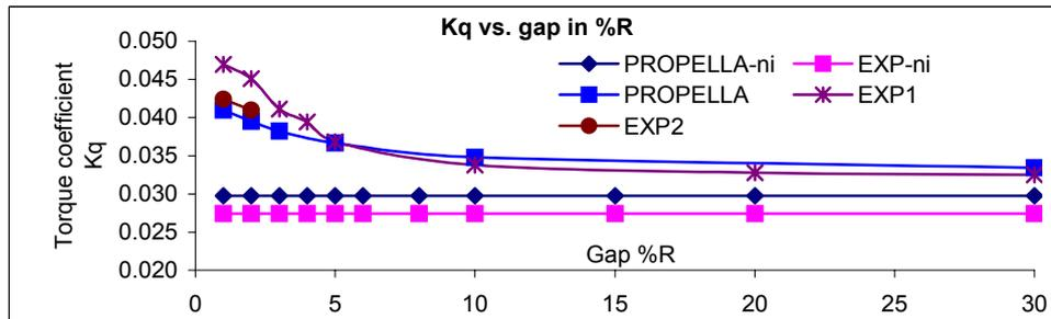
Figure 5: Two sets of comparisons on shaft torque coefficient: one for open water and another for the proximity condition
