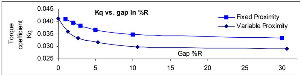
Figure 7: Comparison of torque coefficient for the fixed proximity and variant proximity computations
