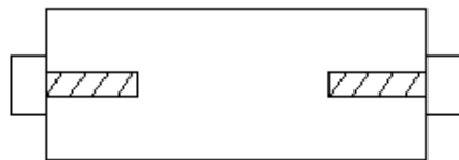
Figure 5: Bushing for wheel that will allow it to rotate
