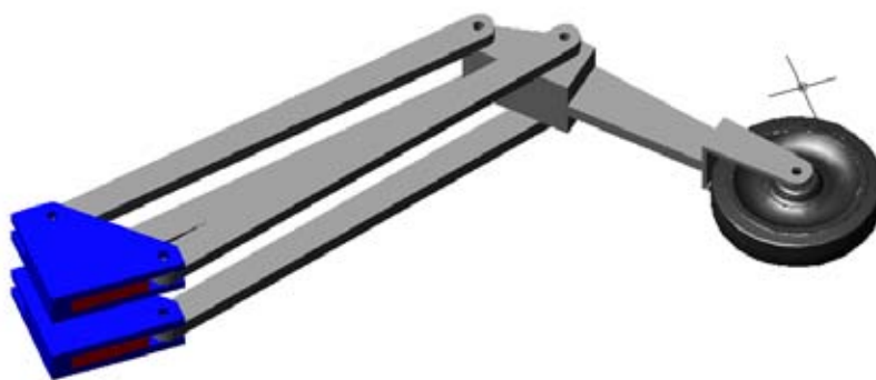
Figure 4: Leg with fork that distributes force evenly
