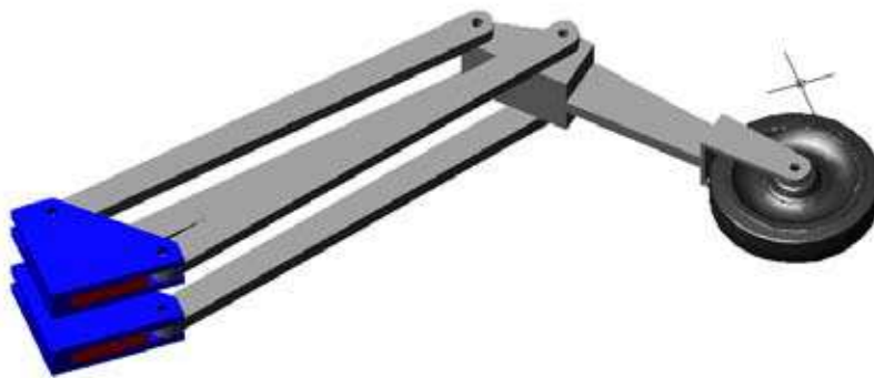
Figure 4: Leg with fork that distributes force evenly
