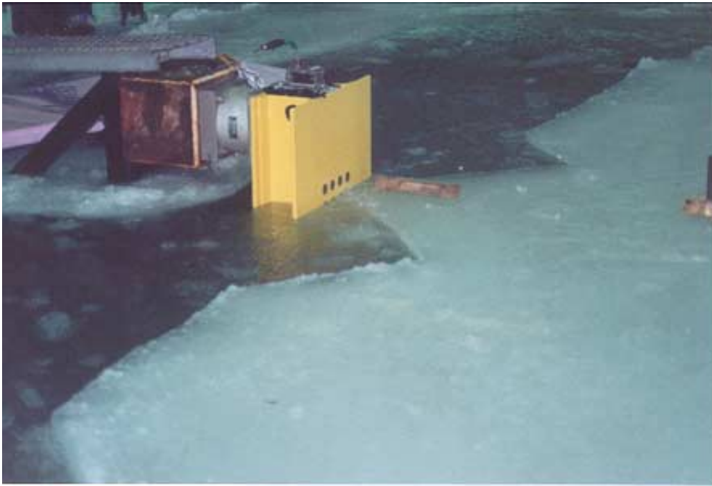
Figure 7 Floe with 90° wedge-shaped edge (#4) impacting test structure
