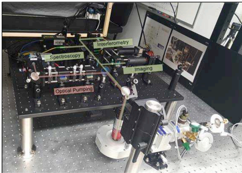
New single photon source measurement apparatus
