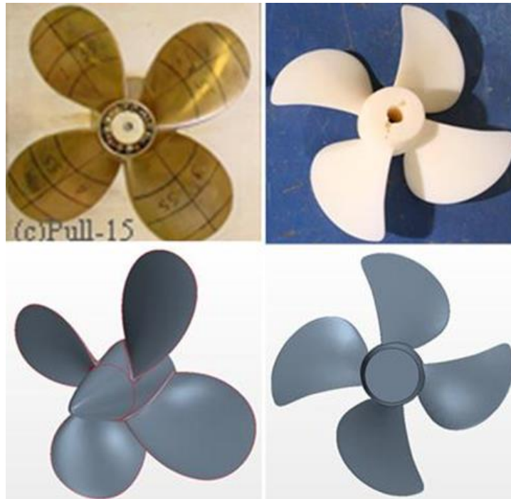
Figure 1: The Base and the Second propellers; Left- the physical and rendered models of the Base propeller, Right- the physical and rendered models of the Second propeller
