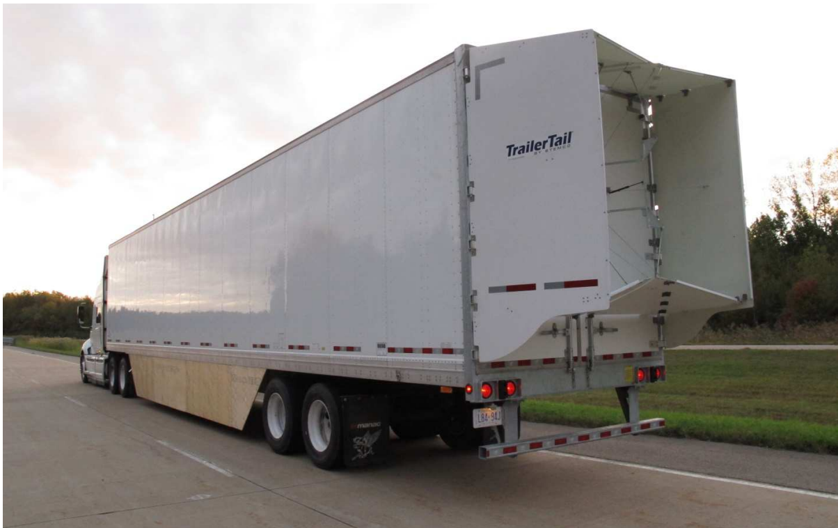
Figure 2.2: Photograph of the trailer configured with side-skirts and a boat-tail.
