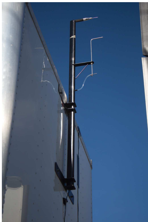
Figure 2.6: Wind-measurement probes mounted to front face of the trailer (Cobra probe - high, pitot-static probe - low).
