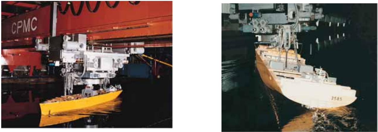
Figure 1: PMM in HSVA Towing Tank. CPMC is computerized planar motion carriage.
