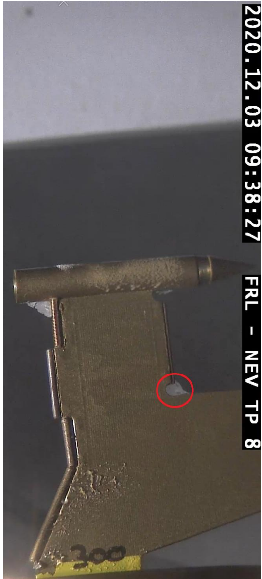
Figure 13. A picture of the Nevzorov probe with icing being seen touching the LWC reference wire during testing.
