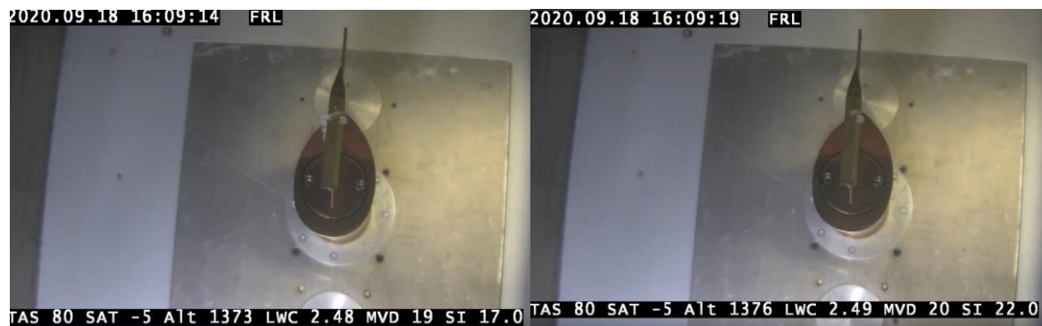
Figure 16. a and b. Photos taken of the sensor before and after a large chunk of ice fell off of the side of the sensor. Depicted is a change in the signal on the reference wires between these two points.
