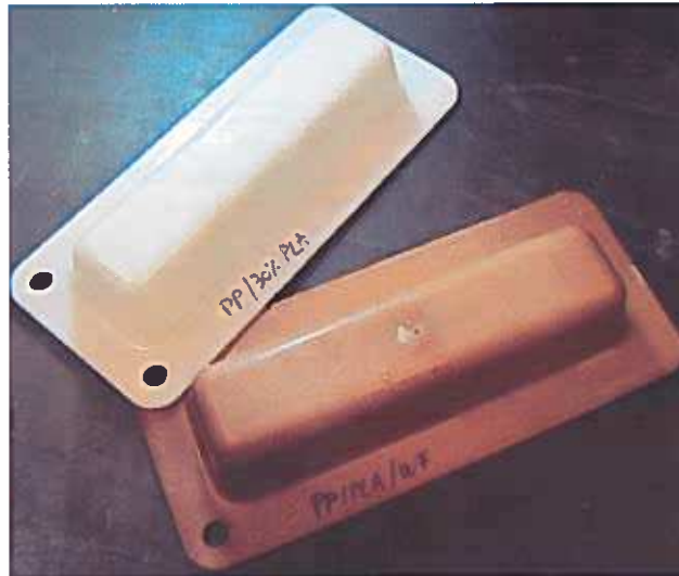
Polyolefins / PLA / cellulosics: injected parts
