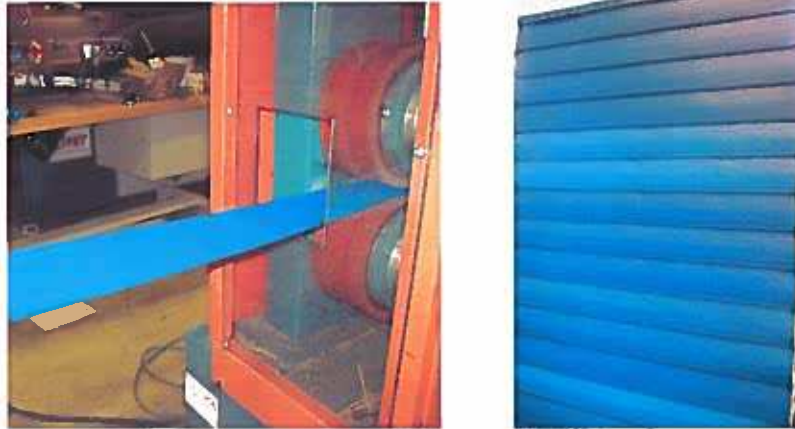
Polyolefins / cellulosics biocomposites: Sidings obtained in extrusion and extrusion foaming
