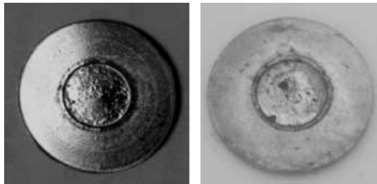
Fig. 4. Circular ^{100}\text{Mo} target before (left) and after (right) irradiation for 1 h with 15 MeV protons at 50 \mu\text{A} .
