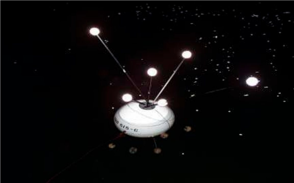
Figure 4: Small Iceberg Model with QUALYSIS Reflectors Fitted
