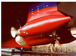
Figure 1: Azipod from ABB, (ABB.com) (reprinted with permission)
