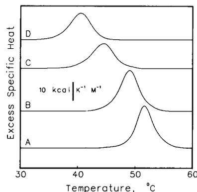
FIG. 4. Differential scanning calorimetric traces for wild-type AKe (A), F86L (B), D84H (C), and G85V (D) mutants. The curves presented were obtained by smoothing raw calorimetric data and subtracting from them the base lines using a cubic interpolation procedure.
