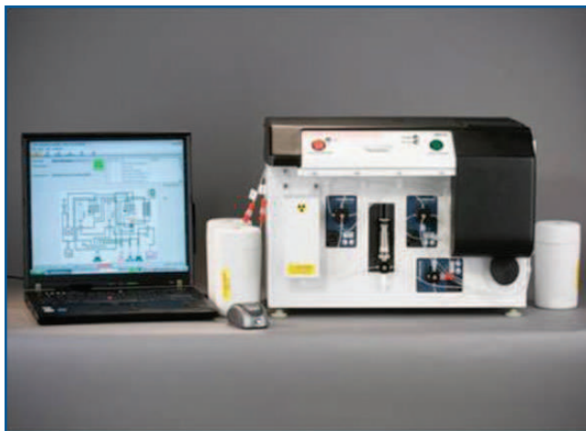
Fig. 4 The Automated Radionuclide Separator (ARSII) developed by NorthStar. The parent solution, in a lead container, is connected to the unit on the left and the product is delivered on the right. A typical run takes about 60 minutes and is fully automated.
