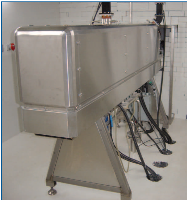
Fig. 3 A Mevex 25 MeV, 25 kW electron accelerator. The machine uses two identical accelerating sections, each fed by an S-band klystron.
