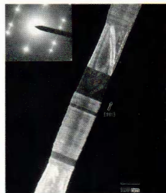
Dark field image of whisker showing twin orientation relationship along length of whisker
