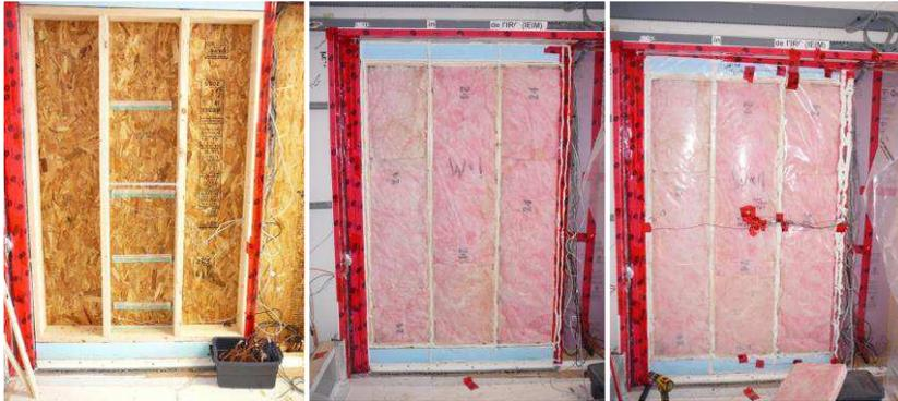
**Figure 6. Wall 1 (XPS) – (i) Stud wall wood frame with OSB, (ii) GF batt insulation in stud cavities, (iii) poly vapour barrier**
