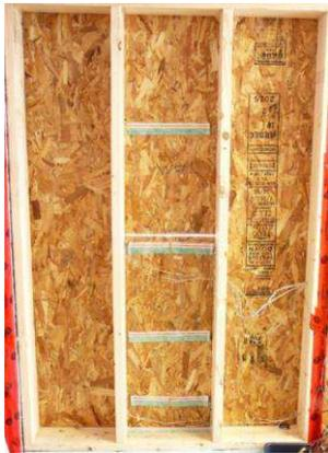
**Figure 12 – W1 : Response of moisture detection strip to the presence of moisture in the wall**
