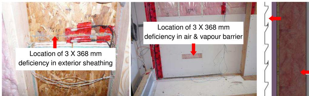
**Figure 10 – Deficiencies in wall test specimens showing location & size of deficiency in W1 (XPS)**
