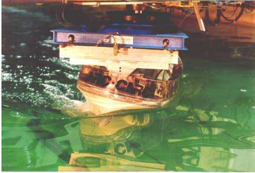
Figure 3, Model tested on PMM (10 knots)
