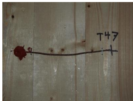
(b) 150 mm wire run along CLT interior surface
