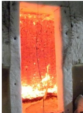
(c) Wall A and ceiling at 60 min
