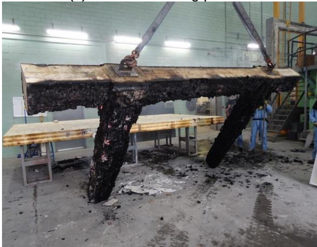
(c) top surface of Glulam beam
