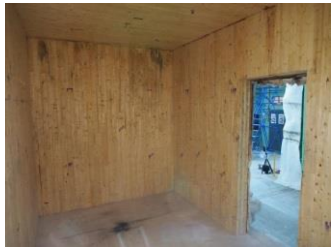
(f) after Test 1 – CLT interior surfaces after cleanup and removal of gypsum board
