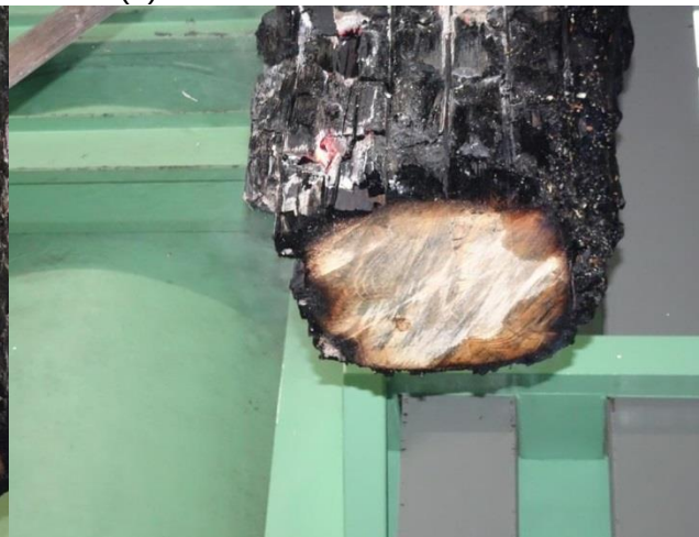
(f) cross section of Glulam column cut
