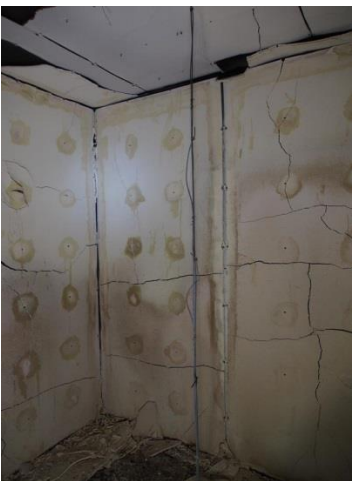
(e) after Test 1 – gypsum board remained: 2 layers on ceiling; 3 layers on walls
