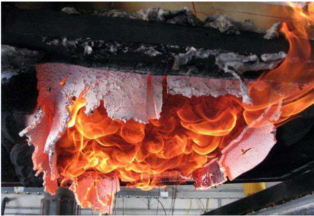
Figure 6: Specimen removal from furnace
