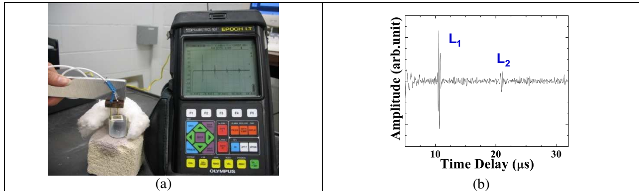
Fig.3 (a) Measurement setup for an IUT made of \text{LiNbO}_3/\text{PZT} composite film at room temperature using an EPOCH LT; (b) Measured ultrasonic data in pulse-echo mode at 800°C.
