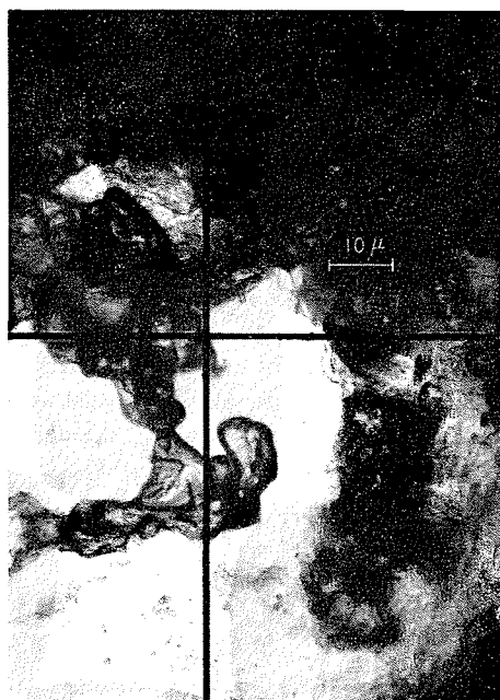
Fig. 10. Photograph of air intrusion into string of pores. The dark areas are air-filled.
