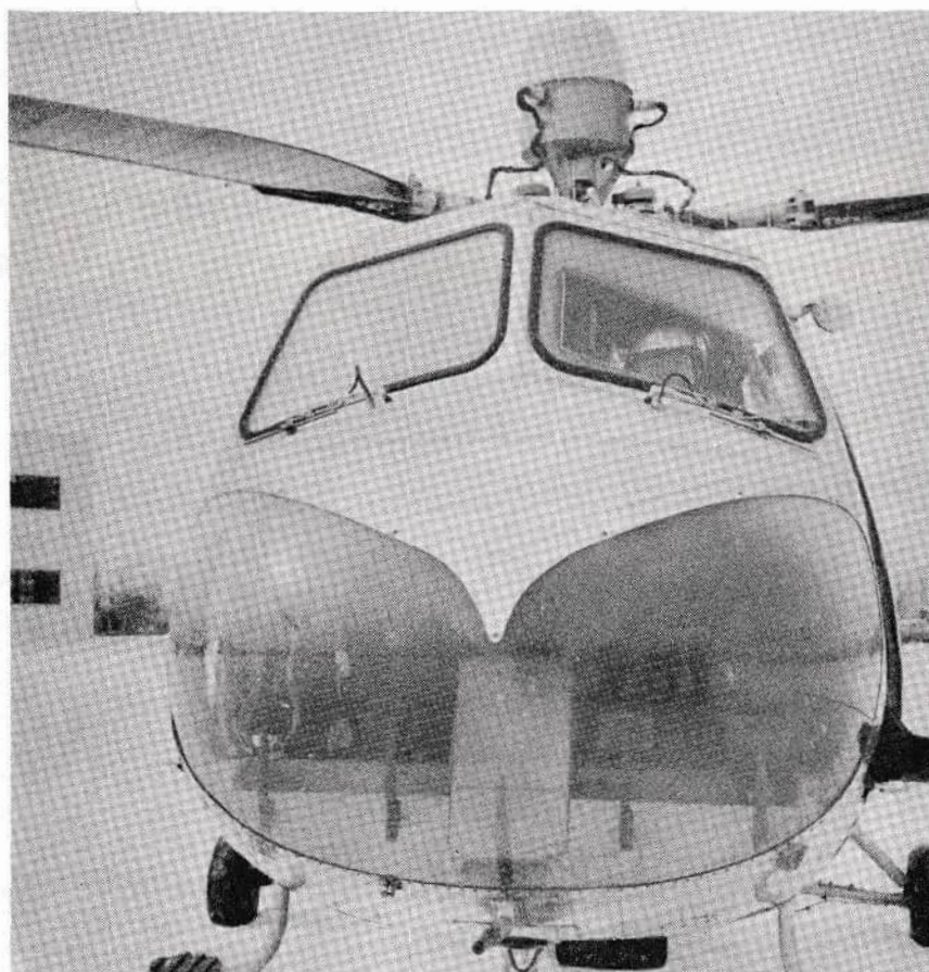
FREEZING RAIN ICE ACCRETION AT 15 M.P.H. T.A.S. SHOWING HEATED WINDSCREEN AREA WINDSCREEN THERMAL ANTI-ICING
