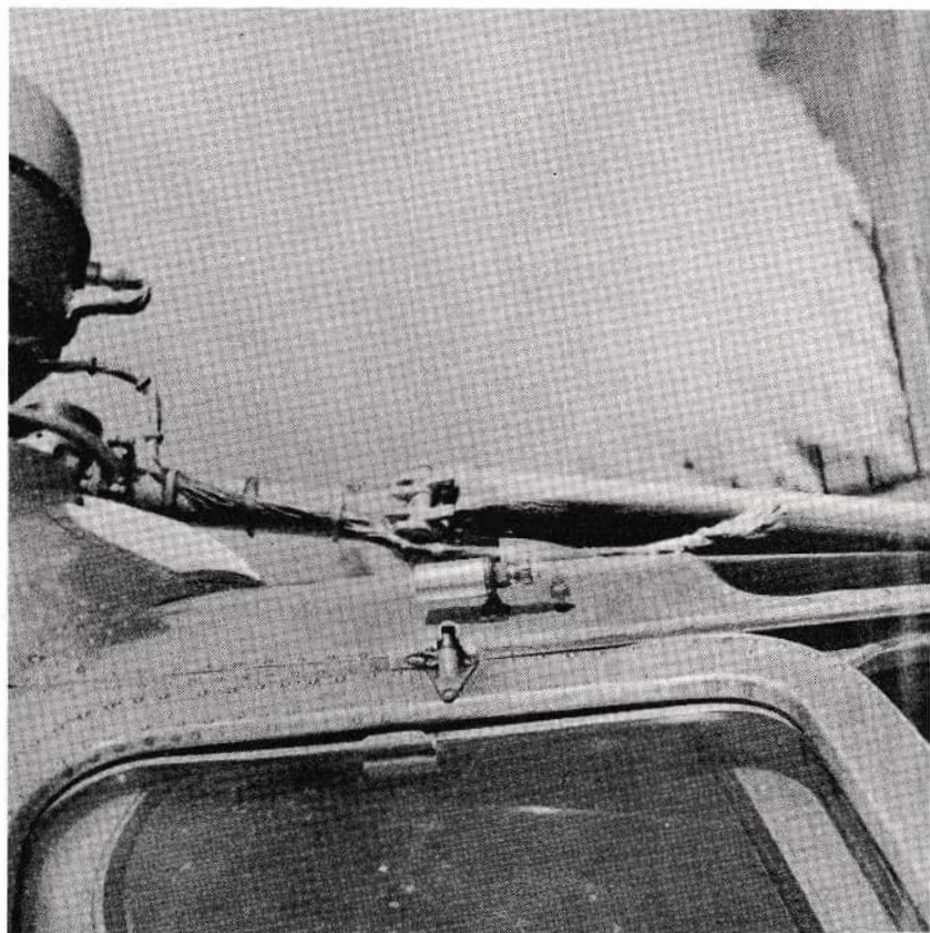
SHIELDED TEMPERATURE BULB ON TOP OF CABIN
