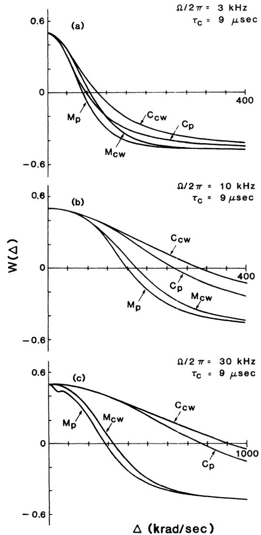
FIG. 1. Normalized inversion  $h(\Delta)$  vs detuning  $\Delta$  for the Gaussian-Markov dephasing model. A correlation time  $\tau_c = 9 \mu\text{sec}$  is assumed. See text for curve descriptions.
