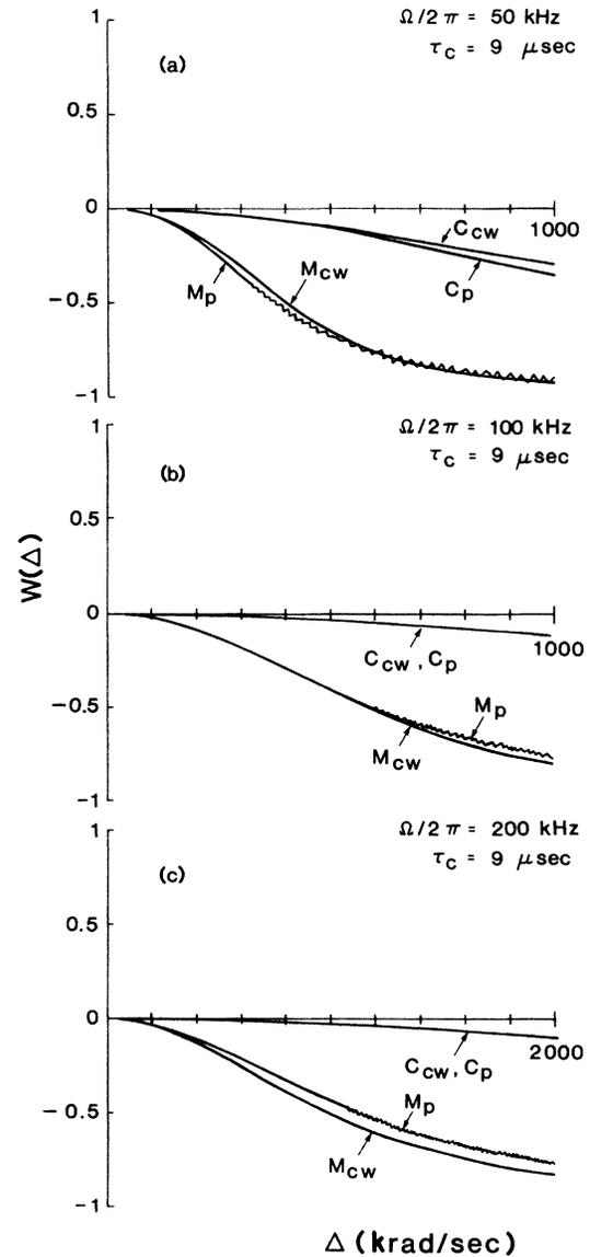
FIG. 3. Unnormalized inversion  $w(\Delta)$  vs detuning  $\Delta$  for the random-telegraph dephasing model at high Rabi frequencies. Correlation time  $\tau_c = 9 \mu\text{sec}$ .
