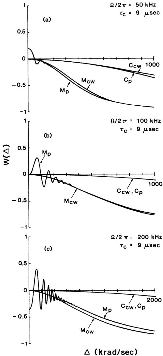
FIG. 2. Unnormalized inversion  $w(\Delta)$  vs detuning  $\Delta$  for the Gaussian-Markov dephasing model at high Rabi frequencies. Correlation time  $\tau_c = 9 \mu\text{sec}$ .
