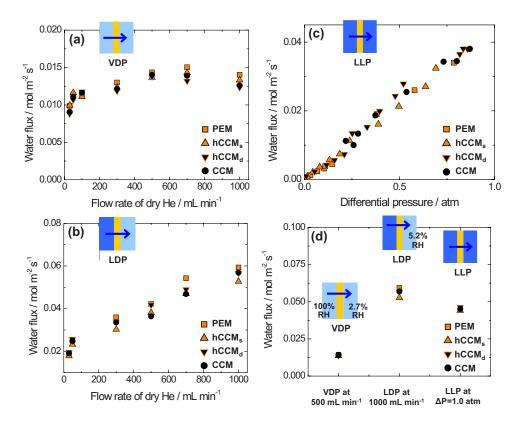
Figure 3. (Color online) Water permeation fluxes through NRE211 and CCMs at 70°C at (a) VDP and (b) LDP as a function of flow rate of the dry helium carrier gas, and (c) LLP as a function of differential hydraulic pressure. (d) Comparison of the representative water permeation fluxes measured by VDP, LDP, and LLP for the NRE211 and CCMs. All measurements were conducted at 70°C. PEM ( $\Box$ ), hCCM<sub>s</sub> ( $\Delta$ ), hCCM<sub>d</sub> ( $\mathbf{V}$ ), and CCM ( $\mathbf{\Phi}$ ).
