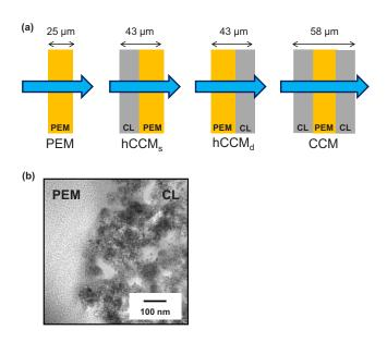
Figure 1. (Color online) (a) Schematic of the NRE211 and CCMs. PEM, pristine NRE211; hCCM<sub>s</sub> (CL upstream of water permeation); hCCM<sub>d</sub> (CL downstream of water permeation); CCM. (b) TEM image of the membrane/CL interface.
