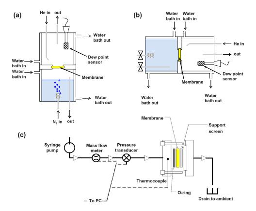
**Figure 2.** (Color online) Schematic diagrams of apparatus: (a) VDP,<sup>10,32</sup> (b) LDP,<sup>10,32</sup> and (c)  $LLP^8$  setups.
