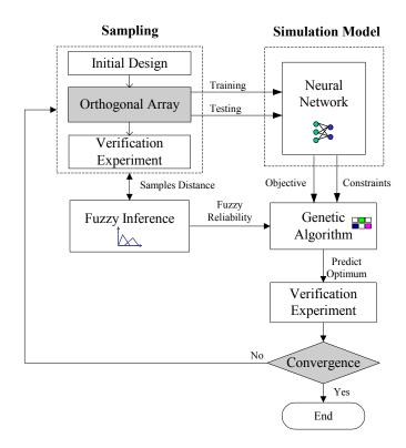
Figure 3 The Optimization flowchart of FUNTGA
