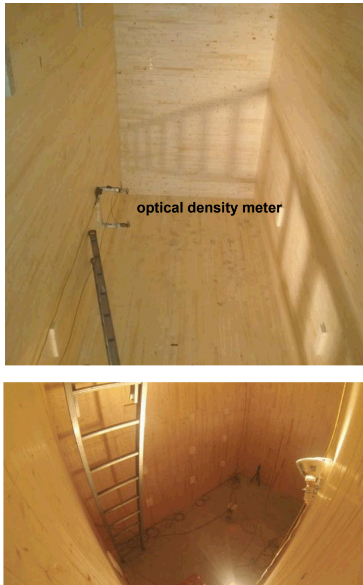
Figure 13. Instrumentation inside the stair/elevator shaft.
