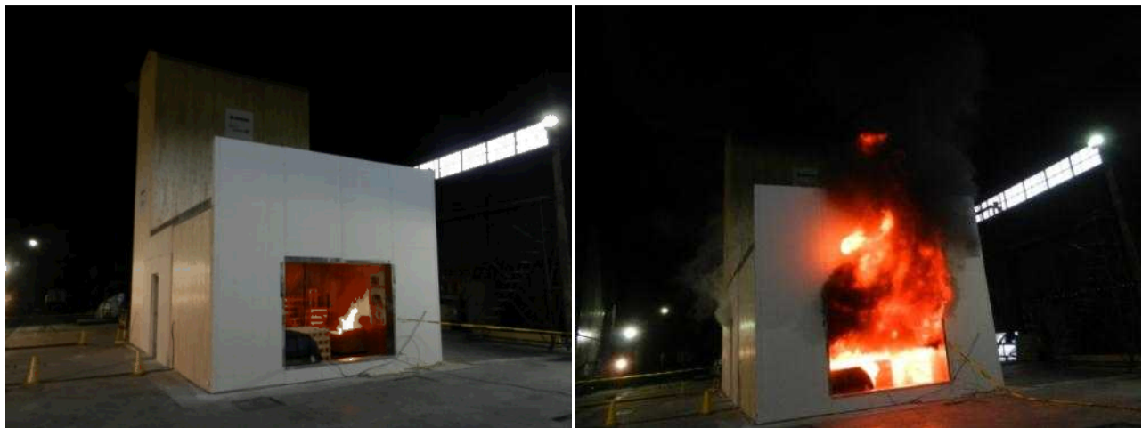
Figure 17. Ignition of the upholstered loveseat followed by flashover at 2 min 35 s.
