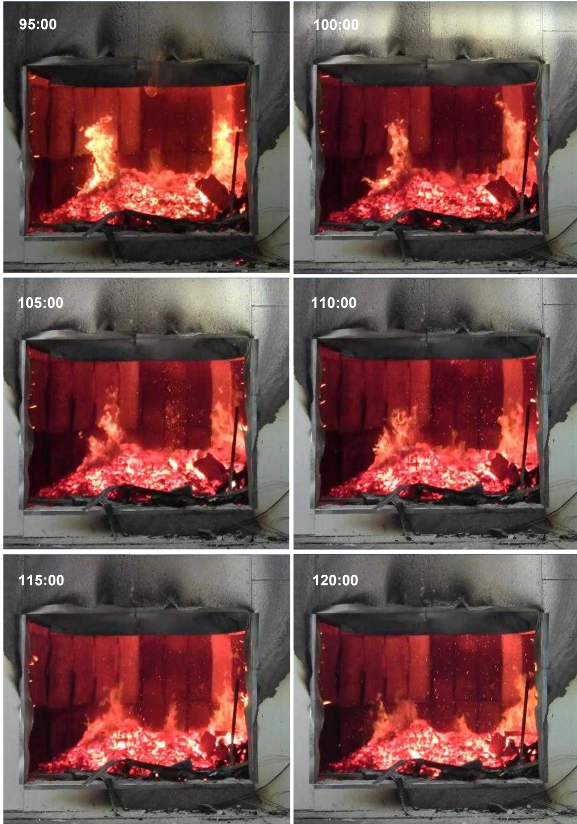
Figure 22. Video graphic captures of fire development (95-120 min).
