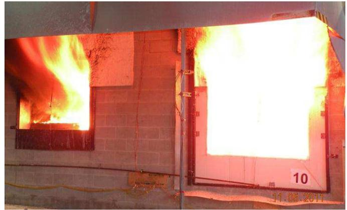
Figure 24. Multiple flashover case (Test PRF-10): Flashover in Zone 2.
