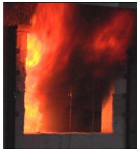
Figure 16. Test PRF-03: Transition to flashover – flames flowing out of entire length of soffit.
