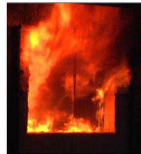
Figure 17. Test PRF-03: All combustible surfaces ignite (flashover: 190 – 270 s).
