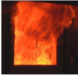
Figure 19. Test PRF-03: Stable post-flashover – flames vigorously flowing and extending out of the window (no visibility inside room).
