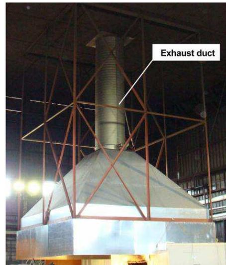
Figure 8. Calorimeter hood and exhaust duct.
