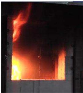
Figure 15. Test PRF-03: Flames flowing out of the top left corner of window (130 – 160 s).
