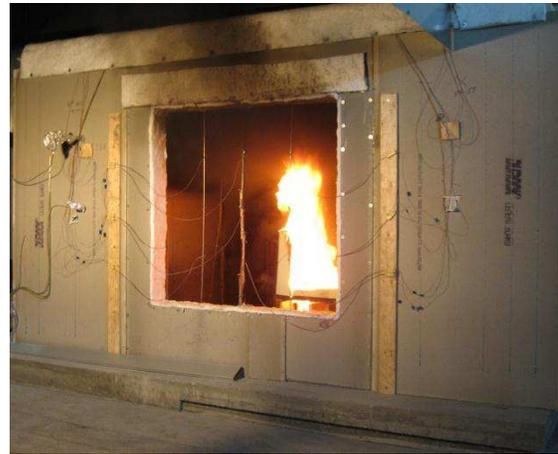
Figure 2. Actual fire experiment in progress in the test room with a window opening of 1,500 x 1,500 mm.
