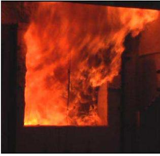
Figure 18. Test PRF-03: Unstable post-flashover (no visibility inside room).
