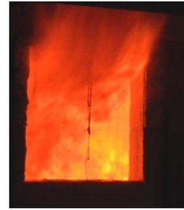
Figure 20. Test PRF-03: Onset of decay phase – flames flowing out with decreasing vigour (inside room becoming visible).
