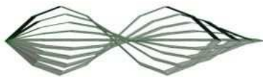
Figure 6: Isometric morph of a simple polygon. The start polygon is a 3D polygon obtained by discretizing the curve y = \sin(x) and by adding thickness to the curve along the z -direction. The end polygon is similarly obtained from y = -\sin x .
