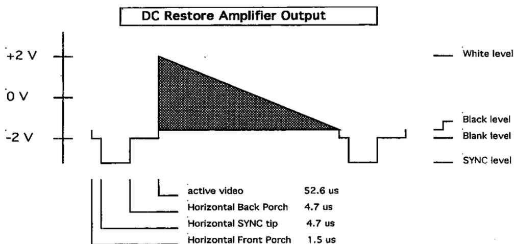
The clamping pulse will be asserted for 3  $\mu$ s in the middle of the horizontal back porch and will clamp the video to the  $-2.0$  V DC level.
