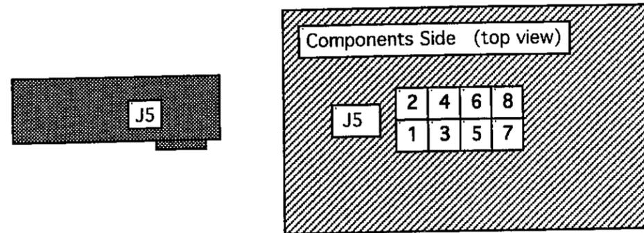
J5 selects one of the three SYNC sources and routes it to the SYNC Decoder. The three possible SYNC sources are the external Analog or TTL composite SYNC or the VIDEO signal output from the 4:1 multiplexer.
