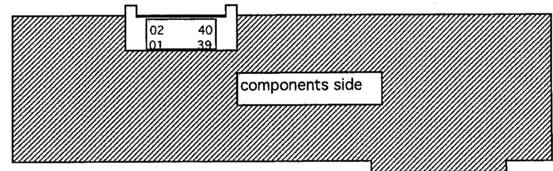
**A6. J11: Camera Synchronization Signals Connector**
