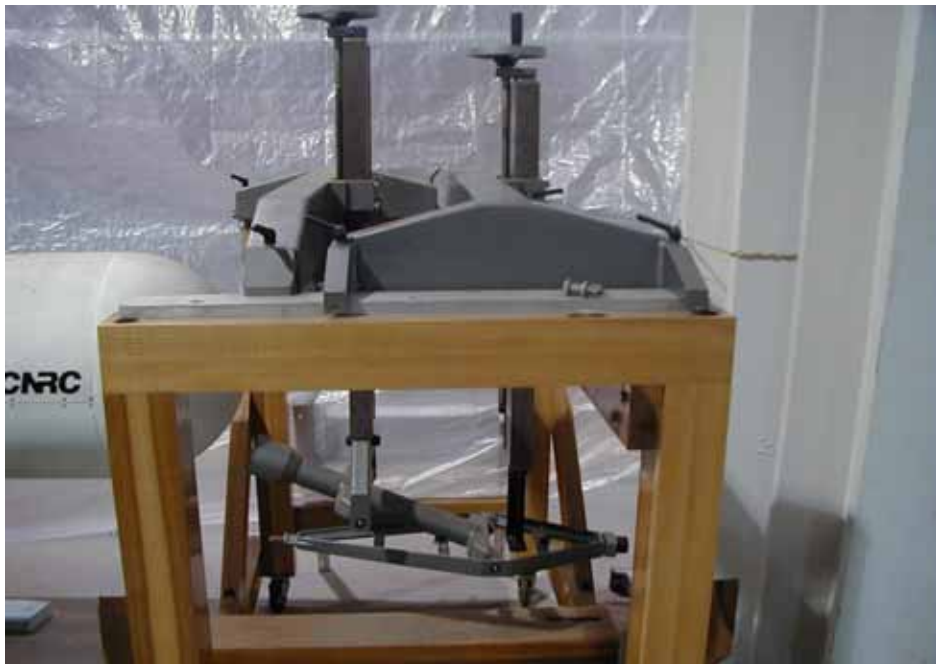
Figure 2. The current yaw restricting "The Grasshopper".
