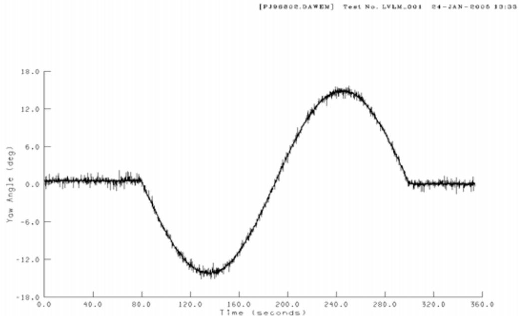
It may be possible to conclude from the above graphs that the yaw rate was not recorded or measured correctly and therefore the yaw rate may not need to be this high in actual testing. The only other yaw rate data that was obtained was from the Terry Fox and the highest rate in those tests was 5.5 deg/s.
