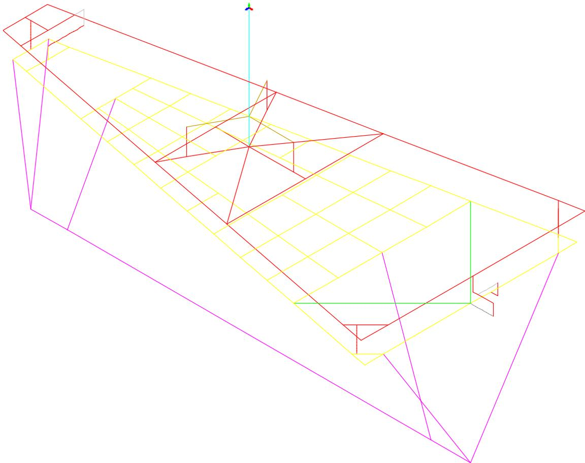
The element model was created in Cadkey . The original wire frame part was used as a template to guide in the placement of center lines for all of the major structural
