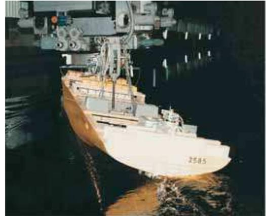
**Figure 1: PMM in HSVA Towing Tank. CPMC is computerized planar motion carriage.**
