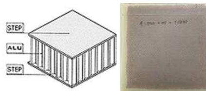
Figure 1. An example of HC covered with two skins of GFRP investigated herein. In this case, the inner defects are unperceivable to the naked eye.
