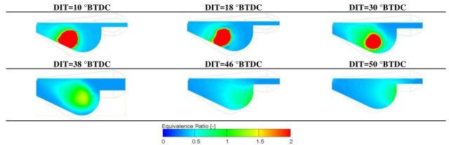
Fig. 4: Spatial contours of total equivalence ratio (at SOC timing) of various diesel injection timings under 25% engine load.
