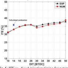
Fig. 6: ITE vs. diesel injection timing for natural gas/diesel dual-fuel mode at 25% engine load.
