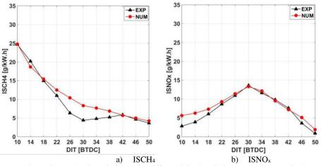
Fig. 7: CH<sub>4</sub> and NO<sub>x</sub> emissions with different injection timings under 25% engine load.
